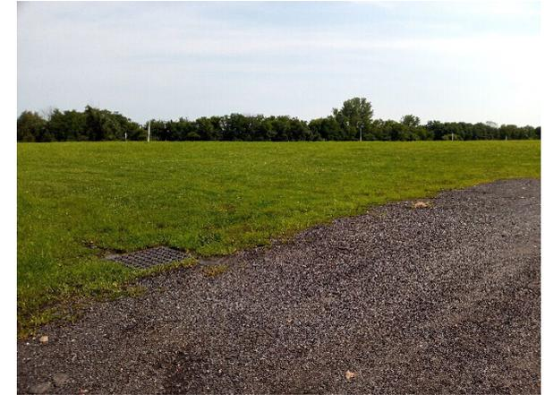
Bioswales can be placed around the roadway to help reduce the existing erosion next to the roadway. At the end of the north bioswale a rain garden can be installed to help promote infiltration of the stormwater prior to entering the existing catch basin. A major portion of the stormwater runoff comes from the capped field which acts as an impervious surface. A preliminary soil assessment suggests that the soils have suitable drainage characteristics for green infrastructure.
