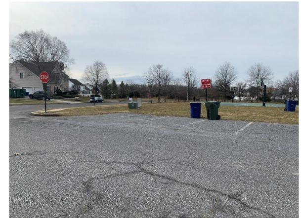
Parking spaces in the south parking lot can be converted to porous pavement to capture and infiltrate stormwater runoff from the parking lot. Rain gardens can be installed alongside the pavement to capture, treat, and infiltrate the stormwater runoff from the parking. A bioswale can be installed alongside the eastern parking lot to help move the stormwater off the parking area. A preliminary soil assessment suggests that the soils have suitable drainage characteristics for green infrastructure.
